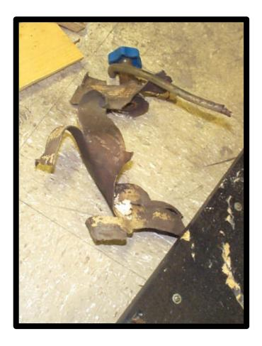
**Ruptured Gas Cylinder**
