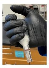
Best practice to properly hold a glass flask when attaching an adapter:
