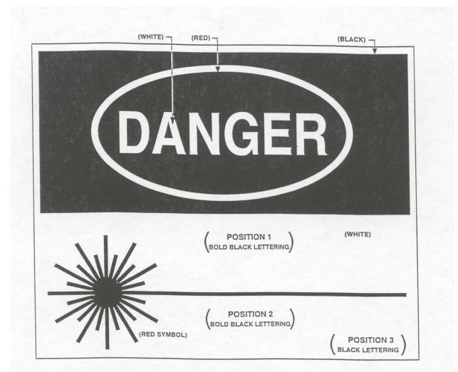
Figure 7. Laser area sign used to designate the nominal hazard zone (NHZ) for Class 3b and Class 4 lasers. Appropriate information must be entered at positions 1, 2, and 3, in accordance with the information presented in Section VII E.
