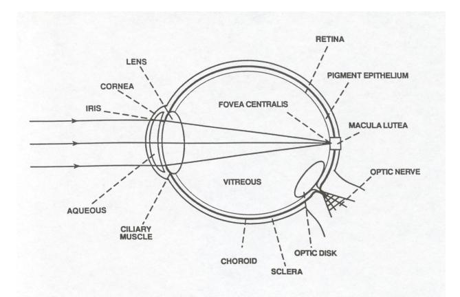
Figure 8. The principal components of the human eye. For laser safety purposes, the cornea, lens and retina are the most significant.
