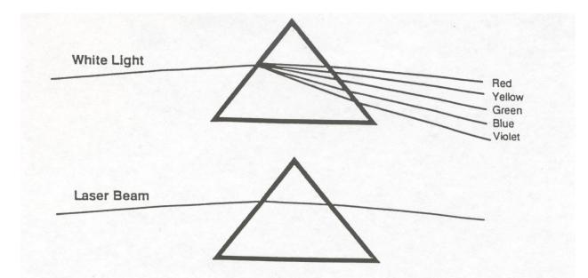
Figure 1. While white light contains all of the visible colors of the spectrum, a laser beam is composed of one color (or wavelength) only. It is this property of laser radiation which facilitates the wearing of laser safety eyewear, which selectively blocks a specific wavelength (or band of wavelengths), and permits sufficient visible light at other wavelengths to pass through to provide adequate visibility.
