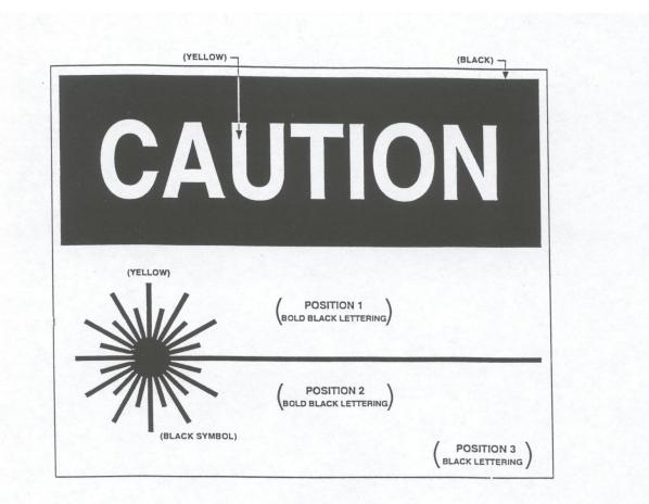
Figure 6. Laser area sign used to designate the presence of a Class 2 laser (rarely) or a Class 3a research-type laser. Appropriate information must be entered at positions 1, 2, and 3, in accordance with the information presented in Section VII E.
