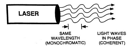
Figure 3. While incandescent light bulbs emit incoherent (not in phase) light at all visible wavelengths, lasers emit light that is both coherent (in phase) and monochromatic (only one wavelength is emitted).
