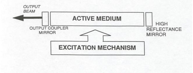
Figure 5. The primary components common to all lasers.
