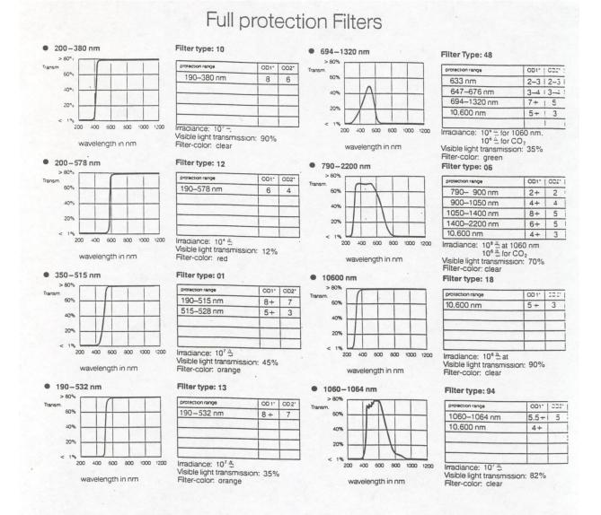
Figure 11. A representation of the type of information provided by laser safety eyewear vendors. Note: OD 1 = optical density before a direct hit; OD 2 = optical density after 10 sec of exposure to the direct laser beam (or 100 pulses) at the specified irradiance levels.
