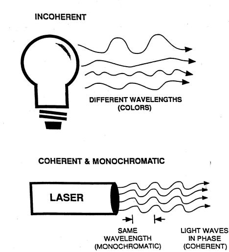
Figure 3. While incandescent light bulbs emit incoherent (not in phase) light at all visible wavelengths, lasers emit light that is both coherent (in phase) and monochromatic (only one wavelength is emitted).
