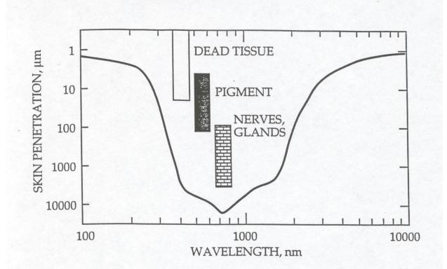
Figure 10. The depth of penetration of laser radiation into the skin, as a function of wavelength. Note: 1000 nm = 1  $\mu$ m.
