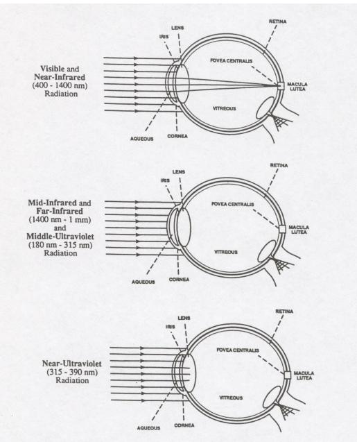
Figure 9. The locations of eye injuries produced by laser radiation, as a function of the wavelength of the radiation. Note: 1000 nm = 1  $\mu$ m.
