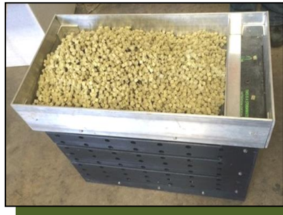
Refilling tray on cartridge with bulk media.
