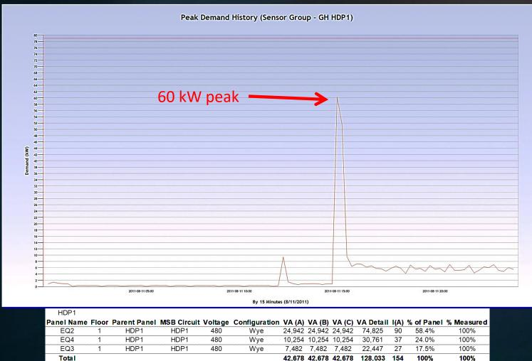
HDP1 is a distribution board on the 1st Floor. It is responsible for feeding several equipment loads, autoclave units EQ2, EQ3, and EQ4. HDP1 is fed directly from the main switchboard at 480/277 volts. The board maximum current rating is 225 amps. The largest load on HDP1 is the medium autoclave EQ2, which is rated at 75kVA.
